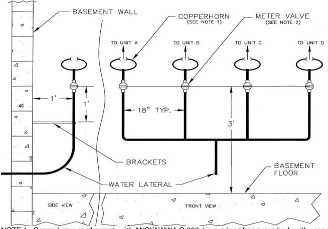
NOTE 1: Copperhorns shall comply with ANSI/AWWA C-800, have a lead free brass body with copper arms and swivel connections manufactured by Ford in the following sizes.
