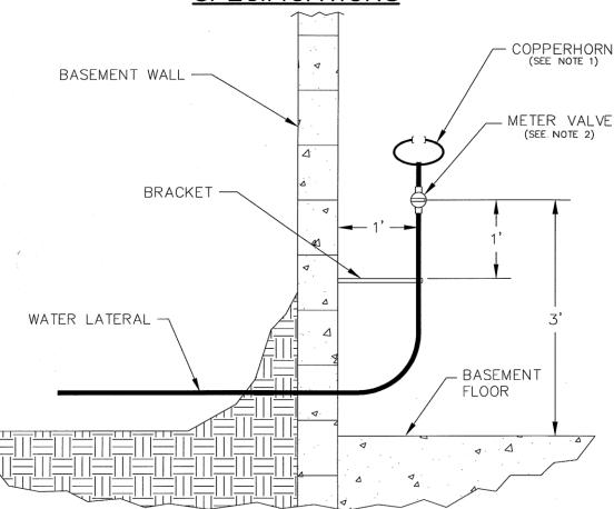
NOTE 1: Copperhorns shall comply with ANSI/AWWA C-800, have a lead free brass body with copper arms and swivel connections manufactured by Ford in the following sizes.
