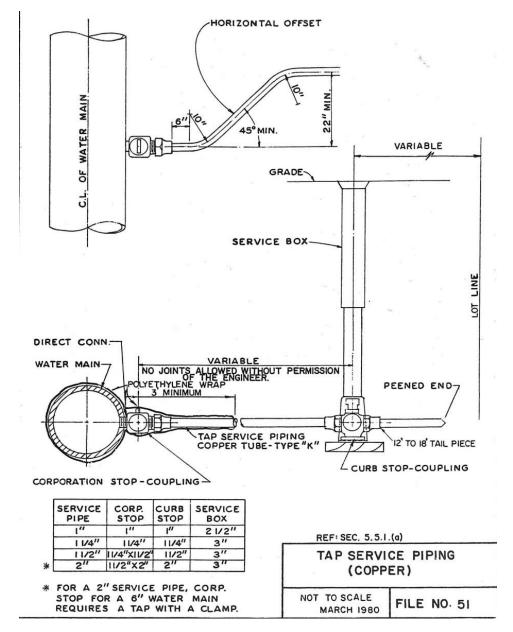
NOTE 1: Curb stops must comply with ANSI/AWWA C-800. All brass must be lead free. All valves must include tracer wire attachment points. The following valves are approved:
