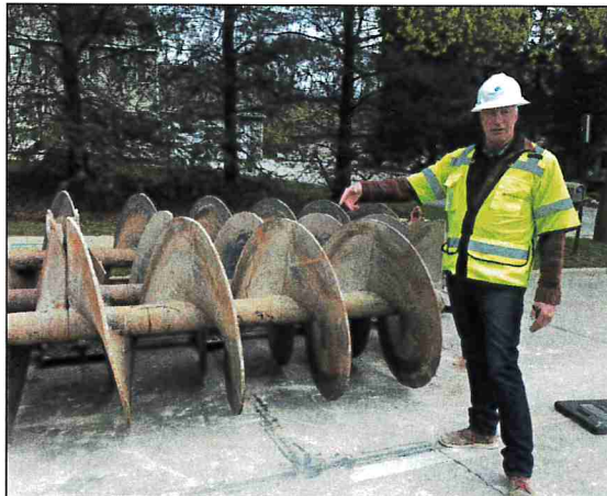
Jim Cobb points to sections of an augur that will be used to drill beneath 124th Street in West Allis.
