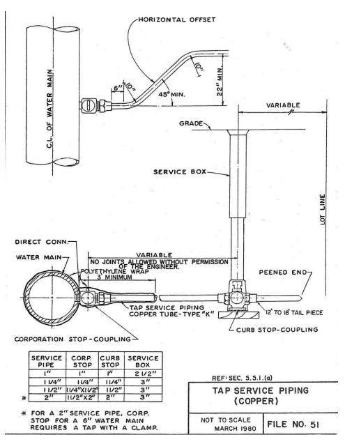
NOTE 1: Curb stops must comply with ANSI/AWWA C-800. All brass must be lead free. All valves must include tracer wire attachment points. The following valves are approved:
